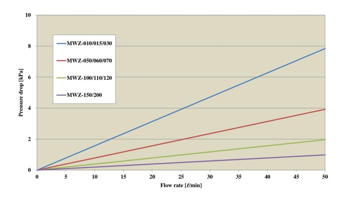
\*\* Fluid: Purified water (20° C) Filter length: 250mm
