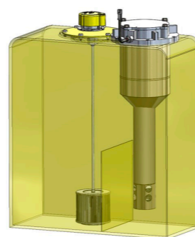
Conceptual drawing of filter case assembly incorporating aeration measures
